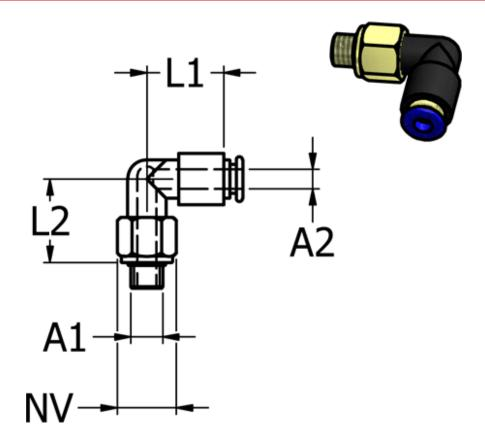
Ext. hose diameter A2 = 6 mm L1 = 16 L2 = 17.2 NV = 10 Thread A! = M5
